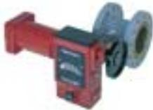
The Masoneilan 30000 Series Varimax control valve provides globe valve type capabilities within a compact rotary style package. Varimax offers a unique flow capacity adjustment feature, which can be externally adjusted in the field to compensate for valve oversizing. This feature can be used to effectively minimize instability in the control loop due to oversizing. Lo-dB trim is available for noise attenuation with higher capacities than equal size globe valves.
